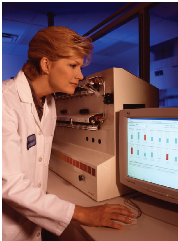
The Virtual Aroma Synthesizer emits a blend of scents that can be mixed in and out in real time.
