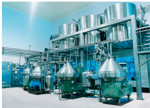
Four juice centrifuges used to reduce pulp level of juice to the desired concentration.
