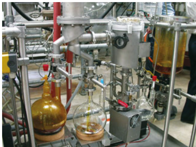
LMR employs rectification, thermal distillation and molecular distillation, slicing materials into distinct pieces and then “reassociating” them, minus undesirable segments.
