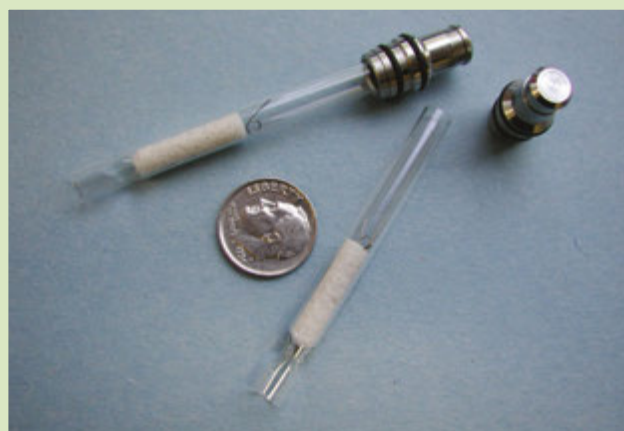
PDMS foam trap in a GERSTEL desorption tube
