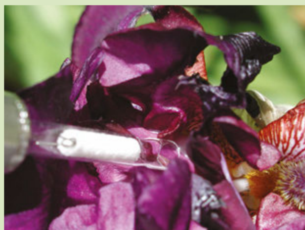
PDMS foam TDU tube inserted into the iris during extraction
