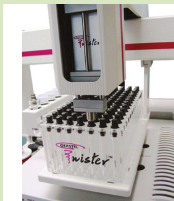
Automated analysis of PDMS foam tubes with GERSTEL TDU and MPS2
