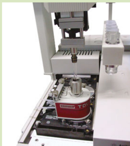
PDMS foam tubes automatically transferred by GERSTEL MPS2 from storage tray to GERSTEL TDU
