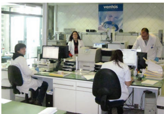
Ventós' quality control lab is equipped with GC/FID and GC/MS and performs organoleptic, chemical and physical analysis of the company's 1,600 materials; the company is ISO-certified for high-volume products.
