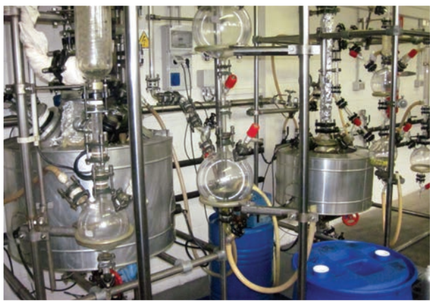
A view of the naturals plant overseen by Viñas; while many of the company's ingredients are steam distilled in-field, short-path molecular distillation takes place in the company's Barcelona site.
