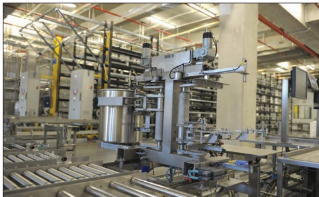
Raw materials are lifted and carried by robots.
