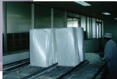
Blocks of menthol from the second stage of crystal isolation standing on a drip table to release the remaining DMO.
