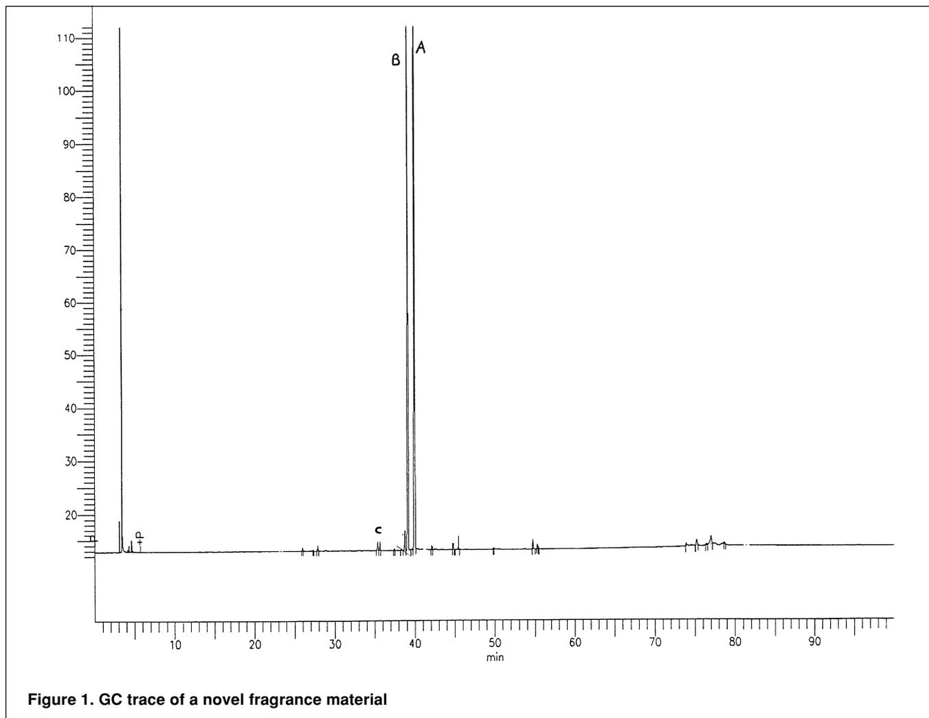
Figure 1. GC trace of a novel fragrance material
