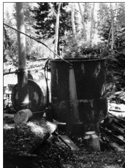
Wood-fired steam boiler and coil condenser housed in cold-stream-fed water tank
