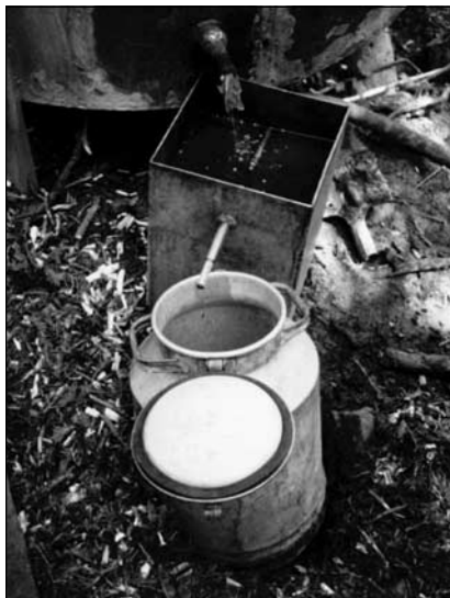
Receiver for condenser steam and essential oil
