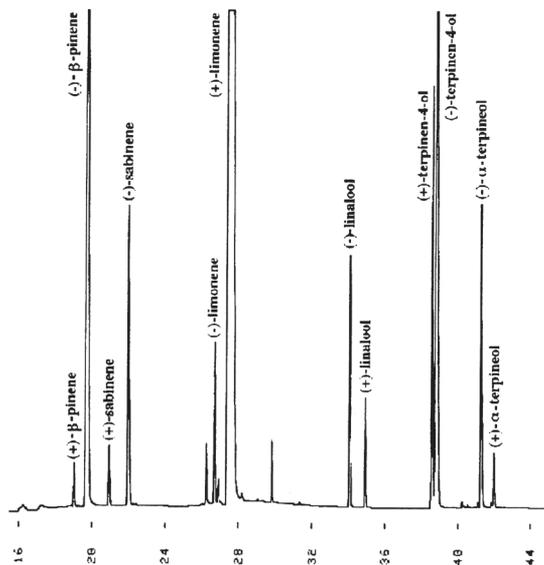
Figure 8. GC chiral chromatogram of the heart-cuts of sabinene + b-pinene, limonene, linalool, terpinen-4-ol, and  $\alpha$ -terpineol of key lime oil type B
