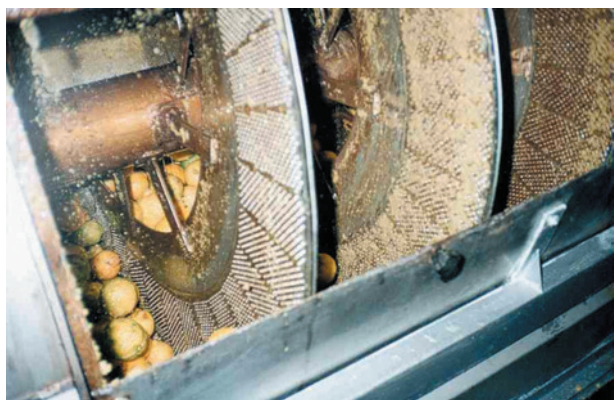
The Pelatrice-style rasper is the third main method of processing, in which the fruit is subjected to rolling disc graters that allow the flavedo to be rasped.
