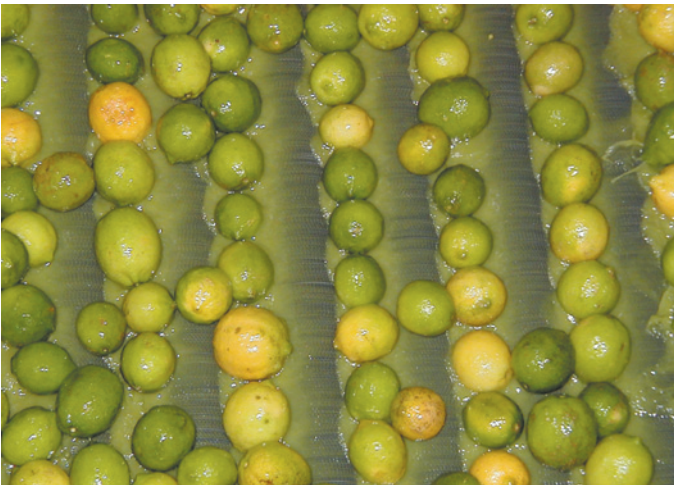
The Brown Oil Extractor (BOE or Brown) process extracts the oil from the fruit first by gently puncturing the flavedo, or peel, of the fruit with thousands of stainless steel needle points.
