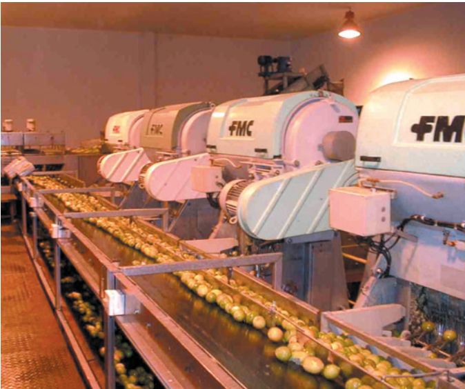
The FMC-type extractor is the most common method used to extract the oil and juice from the lemon.
